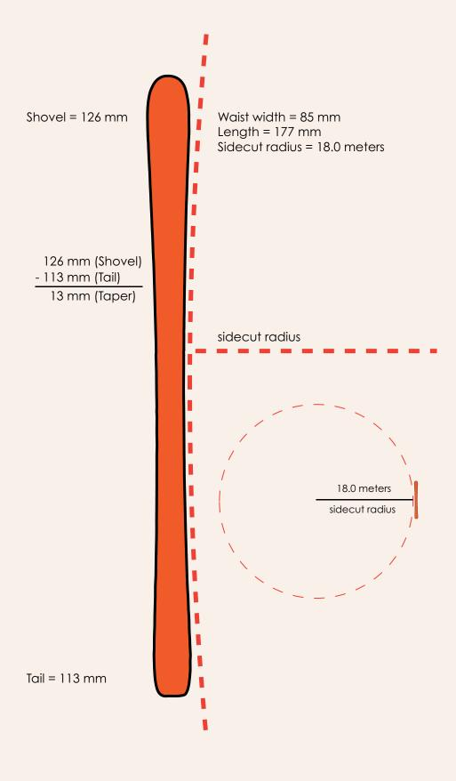
Figure 1. Sidecut radius and taper
